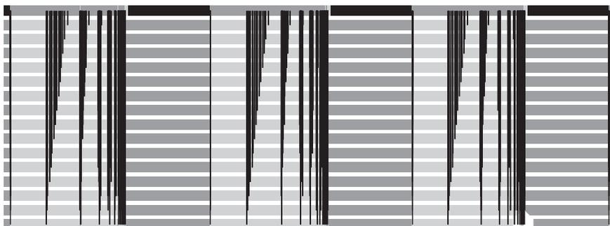
**Figure 15.7** Gantt chart covering 7.16 s of optimization cycles, that is, PEst steps (ii)–(v), with the nonparallelized step (v). The dark parts identify the duration consumed by executing PEst step (v). In the master (first line), the dark gray areas depict step (ii) and black areas depict step (v). Steps (iii) and (iv) are located in the light gray area between steps (ii) and (v). Vertical arrows represent communication events.
